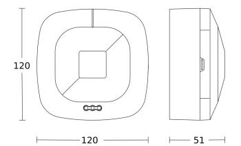
Possible mounting height: 2,50 m – 3,50 m Orange: radial and tangential
